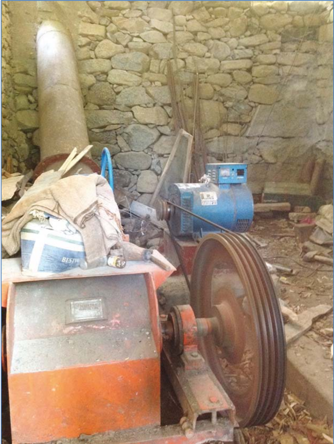
Figure 29: Water mill converted to hybrid system – water mill and hydropower plant in Miandam
