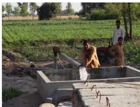
Walayat Ali Using Biogas to run Peter Engine for Irrigation of Crops
