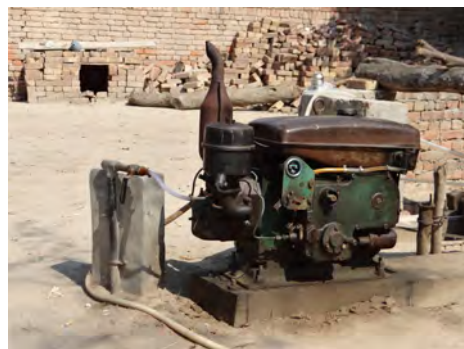
16 Horse Power Diesel-Engine Shifted on Biogas
