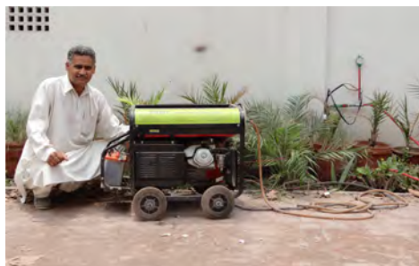
Mian Irfan-ul-Haq Using Biogas to run 5KV Electricity Generator
